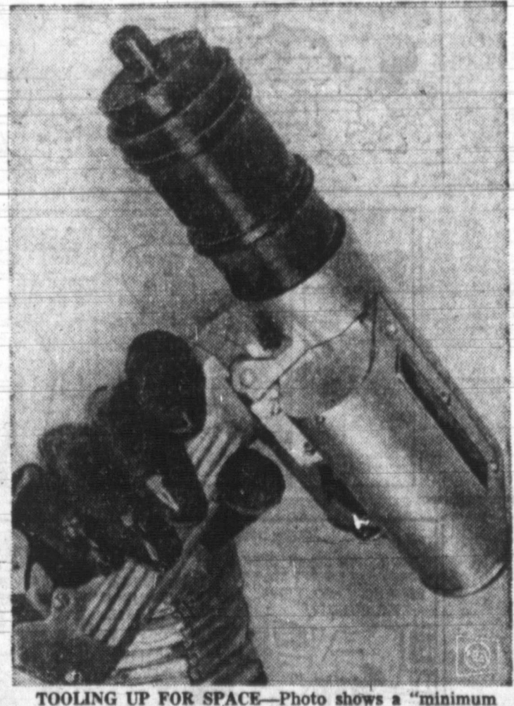
TOOLING UP FOR SPACE—Photo shows a "minimum reaction" power tool recently devised for astronauts engaged in capsule repairs or in setting up space stations while orbiting the earth. Tool overcomes the physical law of action-reaction which prevents conventional tools, such as wrenches, saws or screwdrivers, from being used under conditions of weightlessness.
