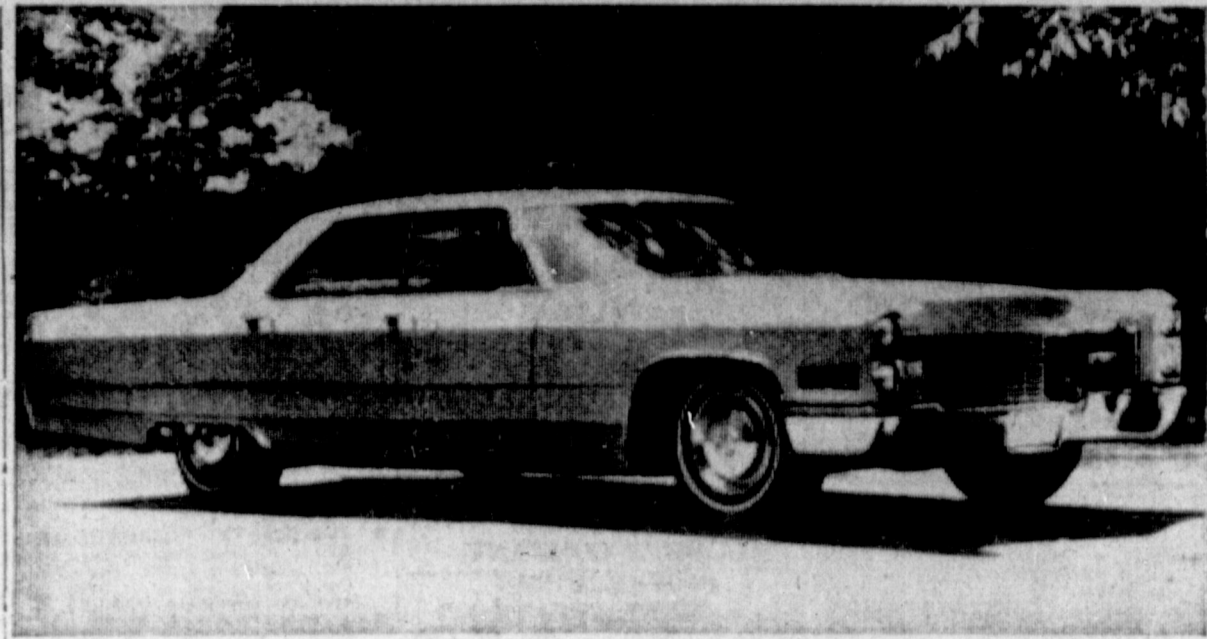
THE BIG CAR —Reduction of chrome and attention to lighting detail is evidenced in this Cadillac Calais Hardtop Sedan. Moldings around the headlamps are finished in body color paint and the popular and practical Cadillac cornering light is fitted into the front fender, adding to the long appearance of the 1966 model. The parking lamps are an integral part of the grille.
