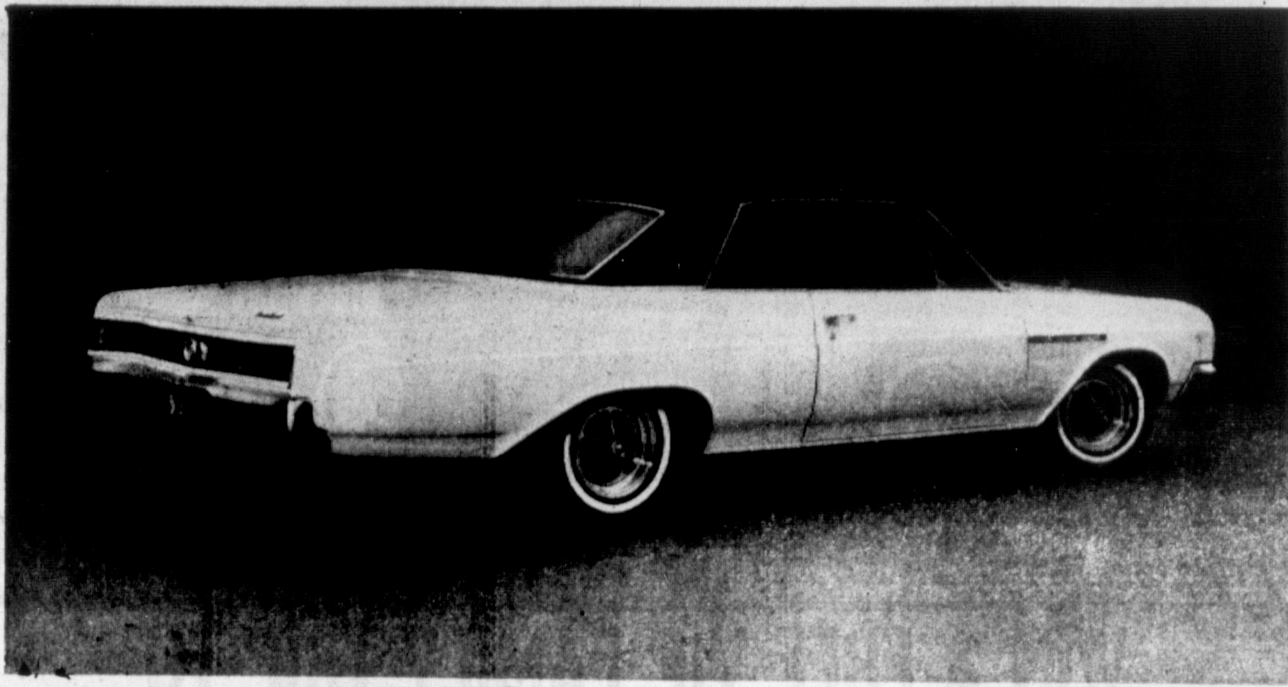
NEW SKYLARK GRAN SPORT — Newest Buick model is this 1965 1/2 version of the Skylark—the Skylark Gran Sport—with new roof and side treatment, plus new ventiports and other features. It's a completely new model—performance-oriented with a V-8 engine of 400 cubic inch displacement that revs up 325 horsepower. To match this performance
