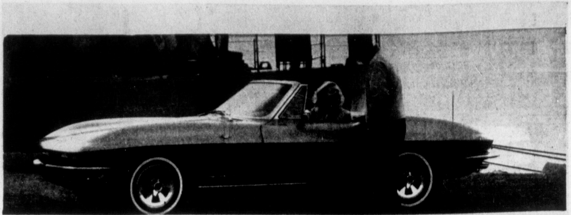
1965 CORVETTE STING RAY CONVERTIBLE — The Corvette Sting Ray registers another first with four-wheel disc brakes as standard equipment for 1965. The new caliper-type disc brakes are virtually fade-free and are self-adjusting. The aerodynamic design of the Corvette's
