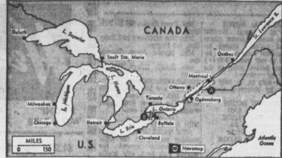
AMERICA'S FOURTH SEACOAST: The St. Lawrence River-Great Lakes waterway extends 2,300 miles from the Atlantic Ocean to Lake Superior. The seaway itself, however, is a 400-mile system of locks, dams and channels from Montreal (A) to the Welland Canal (B) which enables ships to by-pass Niagara Falls. Ships are lifted 602 feet from sea level to Lake Superior.
