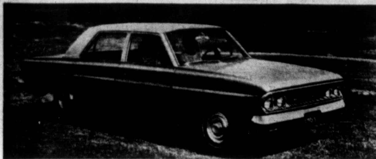
NEW RAMBLERS FOR 1963 — The 1963 Ramblers look much longer with their all-new styling, but actually are more than an inch shorter than past models. Overall height is reduced three inches without sacrifice of interior room. Wheelbase is increased to 112 inches. A new body construction technique is used on the '63 Ramblers for the first time. Curved side glass is standard on the 1963 Rambler, the only low-priced car to have this custom feature. Shown is the Rambler Classic 770 four-door sedan. The new Ramblers are now on display at Tex Evans Buick-Rambler, 124 N. Gray.
