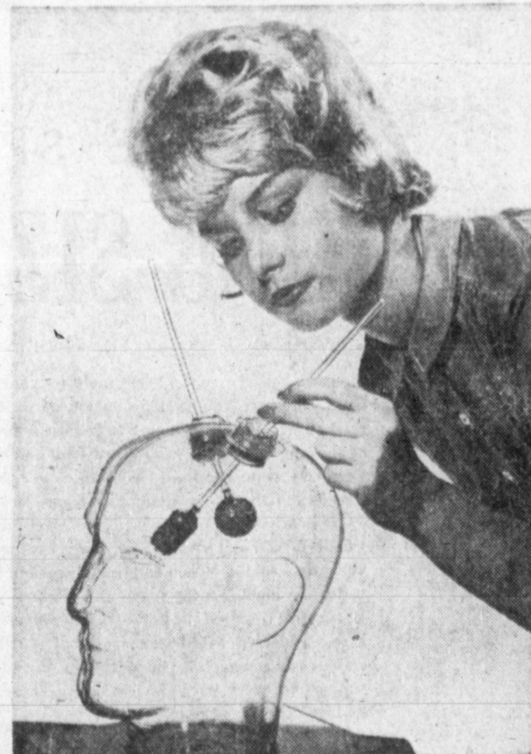
SKULL PHANTOM —A technician in a White Plains, N. Y., laboratory pre-tests the effectiveness of nuclear radiation scanning devices in detecting brain tumors. This device approximates radiation absorption of the human head during examinations.
