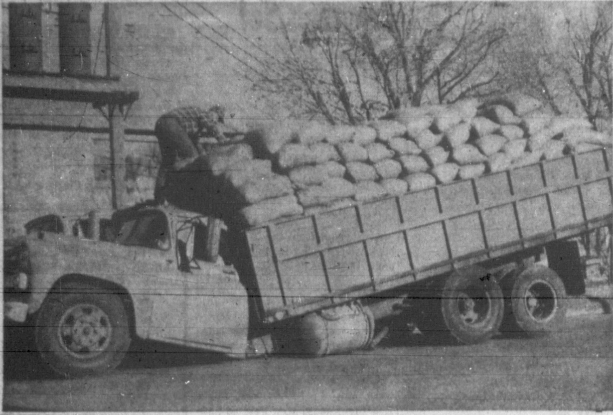
BROKEN BACK —This bob-tail truck loaded with 24,000 pounds of cotton seed cake, was traveling West on Brown St. early Saturday when both sides of the frame, collapsed, leaving the truck in this unusual position. Driver of the truck, L. C. Merdith, Sunray, who is on top of the truck, said he was hauling the feed for cattle from Twitty to Sunray when the accident occurred. He was not injured.
