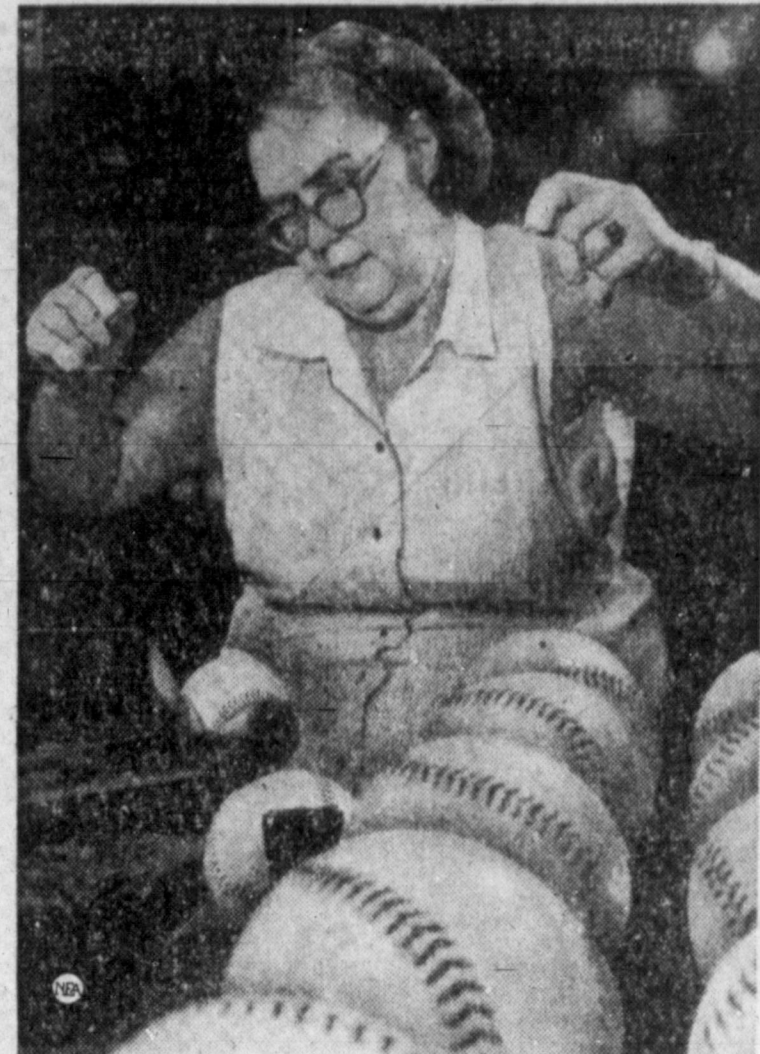
SOURCE OF POWER—In the renewed arguments about the lively baseball, the consensus is that the difference is in the stitching. Beryl Gauthier sews covers on balls at the main A. G. Spalding & Bros. plant at Chicopee, Mass.
