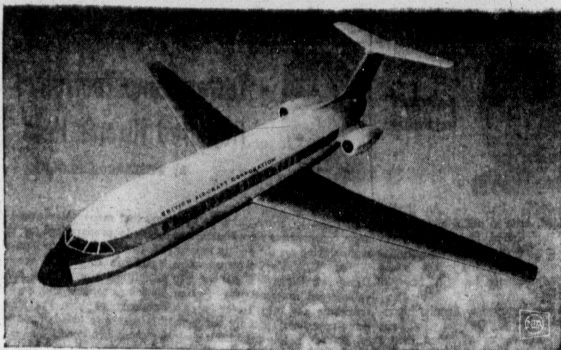
BRITISH JET — A new jet airliner, the BAC One-Eleven, shown in drawing above, is now being built by the British Aircraft Corp. Powered by two rear-mounted turbofan engines and designed for short haul work, the aircraft will cruise at 540 m.p.h., and carry up to 60 passengers.
