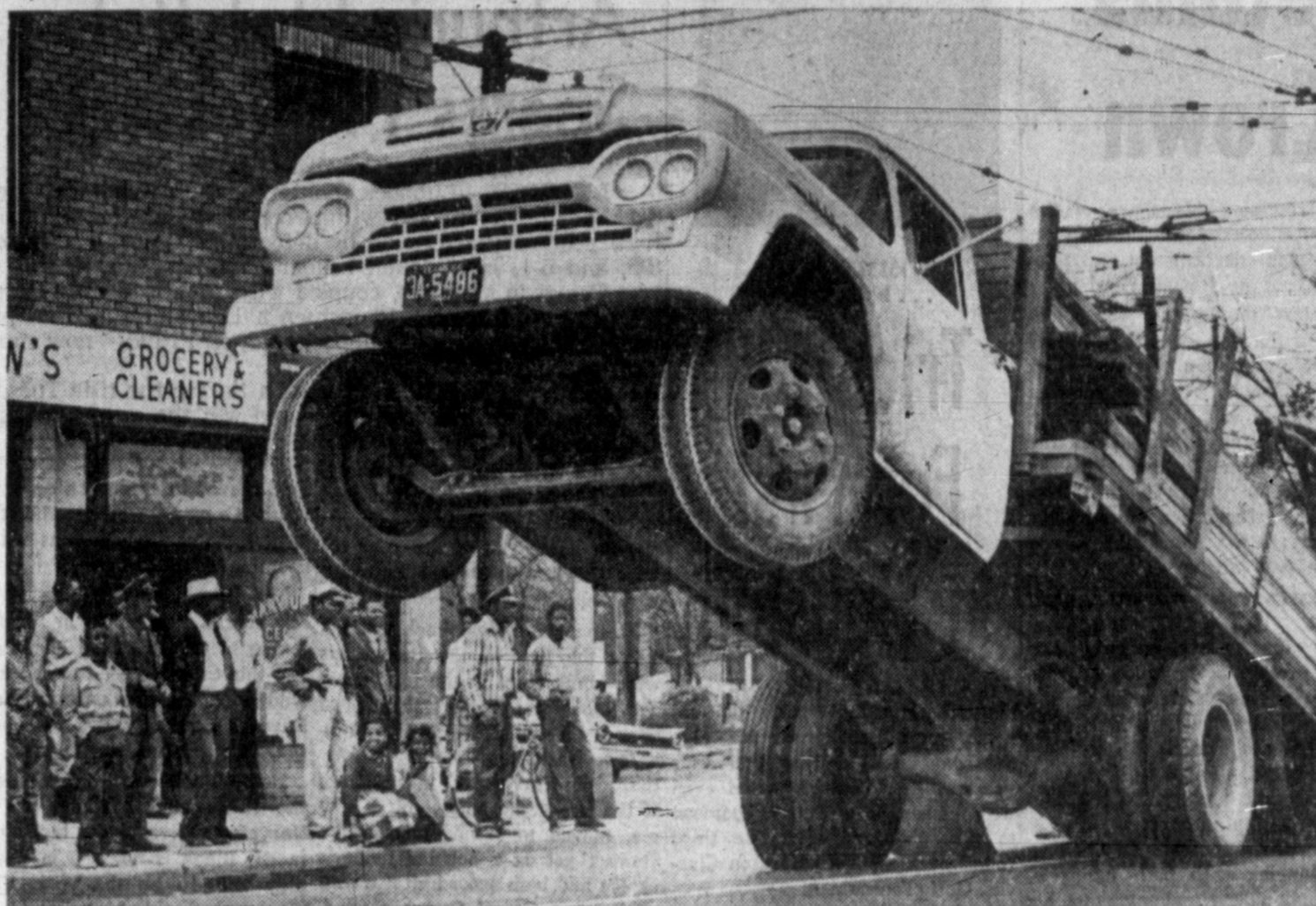
READY FOR TAKE-OFF? —Turning a street in Dallas, Tex., into a kind of launching pad, this lumber truck looks about ready to shoot up into space. Actually, it's just waiting to be rescued by a tow truck. When the driver shifted gears to turn a corner, his load of 18-foot-long lumber slid backwards, which threw the truck out of balance and left it in this embarrassing position. At least it gave the people on the corner something to look at.
