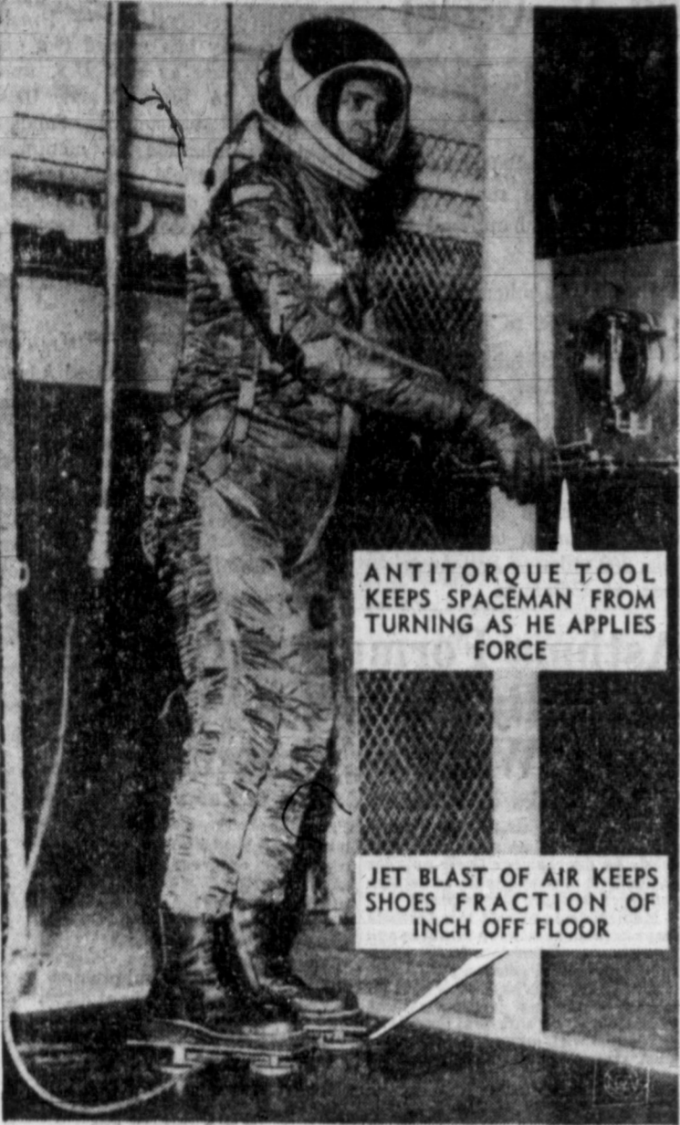
SPACE SLIPPERS —Literally floating in air, engineer Carl R. Adams of Chance-Vought Astronautics Division tests a special tool for use by spacemen. He uses a "plench"—a combination pliers and wrench—designed to prevent a crewman from spinning around as he makes repairs to his ship in weightless space. To simulate weightlessness, Adams stands on a cushion of air while he studies his reaction with no friction to keep him in place.
