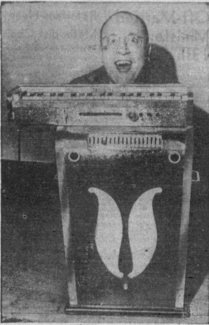
JACK OF ALL NOTES —flappy man is Jean Jacques Perrey, a Parisian who sounds off in New York on the Ondioline, a 44-pound electronic device that looks like a hybrid piano-cash register and sounds like any number of musical instruments. The Ondioline, which has a three-octave keyboard, can be made to sound like a tuba, trombone, clarinet, trumpet, bass fiddle or cello—but only one at a time.
