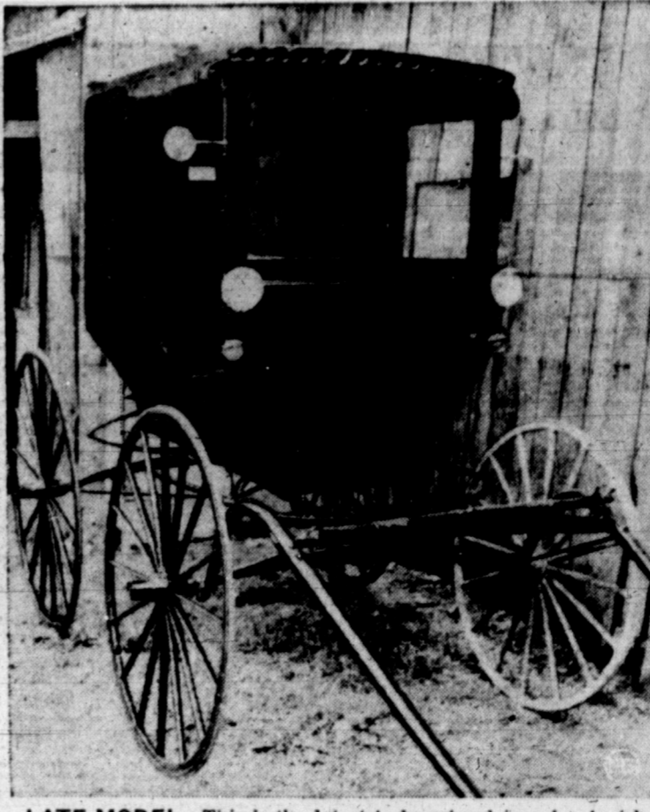
LATE MODEL —This is the latest in buggies driven by Amish in Ohio. It has rear view mirrors, headlights, parking lights and taillights. The buggy costs $500 new, has a battery for the lights. A new state law will require in addition a flashing red light to warn motorists.
