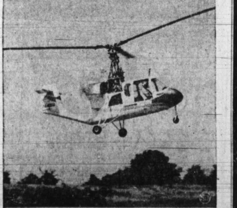
HIGH JUMPER—Able to leap vertically into the air and land the same way, and called simpler and safer to fly than a helicopter or a conventional airplane, the Umbaugh-18 rotary wing aircraft is being put through tests leading to production early next year. Essentially an autogyro, the two-place craft gets its lift from a free-spinning rotor as it is driven forward by a pusher propeller. On take-off, however, power can be applied to rotor, enabling the ship to jump 15 feet or more straight-up.
