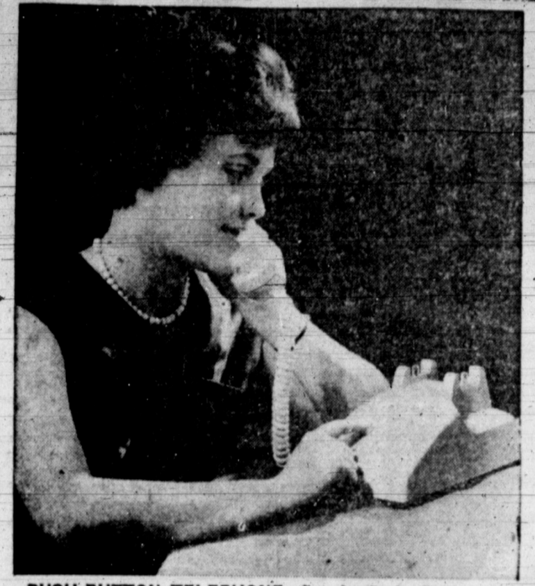
PUSH-BUTTON TELEPHONE —Comely Gayle Grebs tries out an experimental push-button telephone in New York. It is under development at Bell laboratories and may eventually replace the usual rotary setup. The arrangement of 10 buttons—one for each digit—consists of three horizontal rows of three each, plus the zero or operator button at the bottom. Push-button dialing takes about five seconds, compared to nine for rotary dialing.
