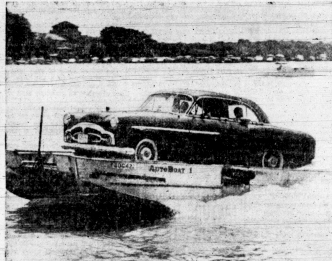
SEA-ING IS BELIEVING —This autobot is equally at home on land or sea, and here it's getting the feel of the bounding main by cruising on the Detroit River. The craft was designed and built by engineer John Brush, who put it together in his garage. The auto powers and steers two airplane fuselage sections which act as pontoons in the water.
