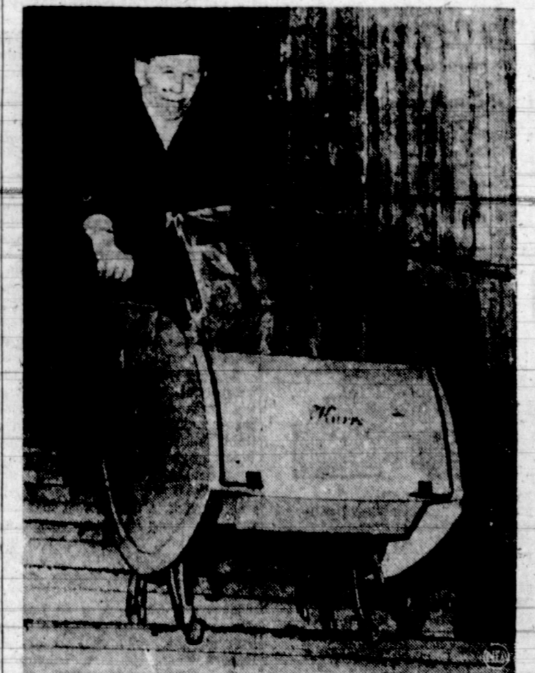
IT WALKS —Since "perambulate" means to walk about, a Swedish inventor has come up with a perambulator that really does walk. As seen above, during demonstration in Stockholm, Wilhelm Peterson's pram has, instead of wheels, 20 metallic feet, fixed to the axle in spoke fashion. It "walks" up and down stairs and, on flat surface, the "feet" impart a rocking rhythm to the carriage, which should act like a lullaby.
