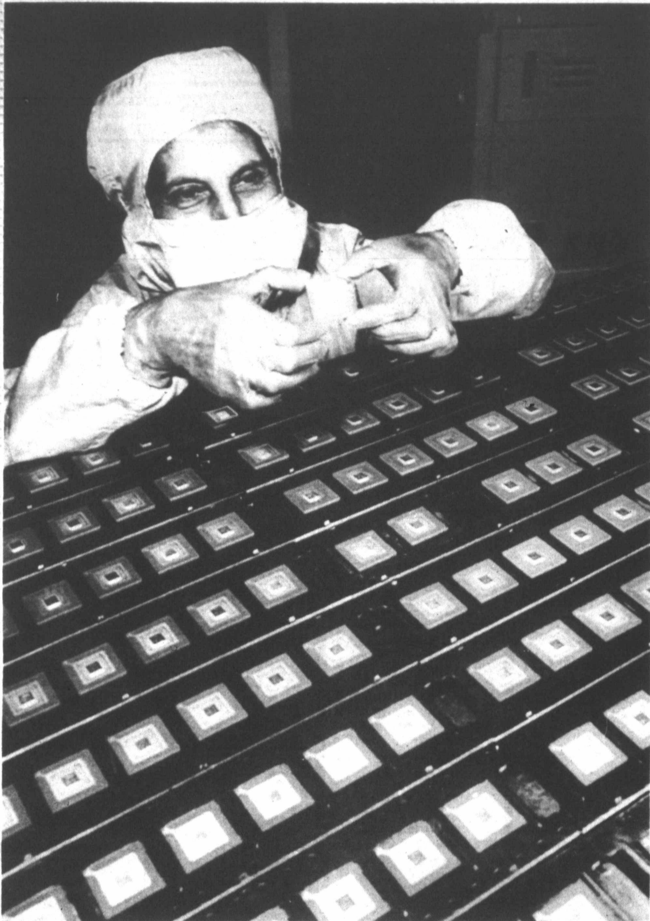
Technician Leonor Soto inspects 68030 50 megahertz electronic chips at Motorola's Austin plant. The chip, used in computers and other electronic applications, offers the equivalent of 250,000 transistors and can process over 10 million instructions per second.
