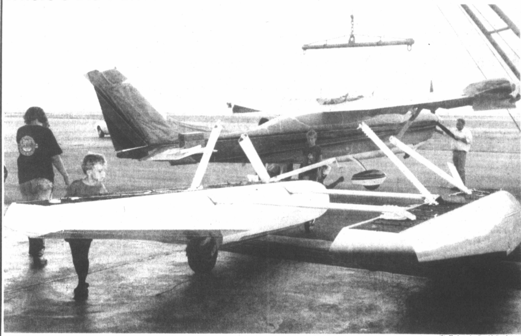
There's not much need for amphibious planes in the Texas Panhandle, even with the rains of this summer, but one was at Perry Lefors Field last week. The plane is being lifted so that its landing gear can be replaced with amphibious pontoon floats. The new floats contain wheels that can be hydro-
