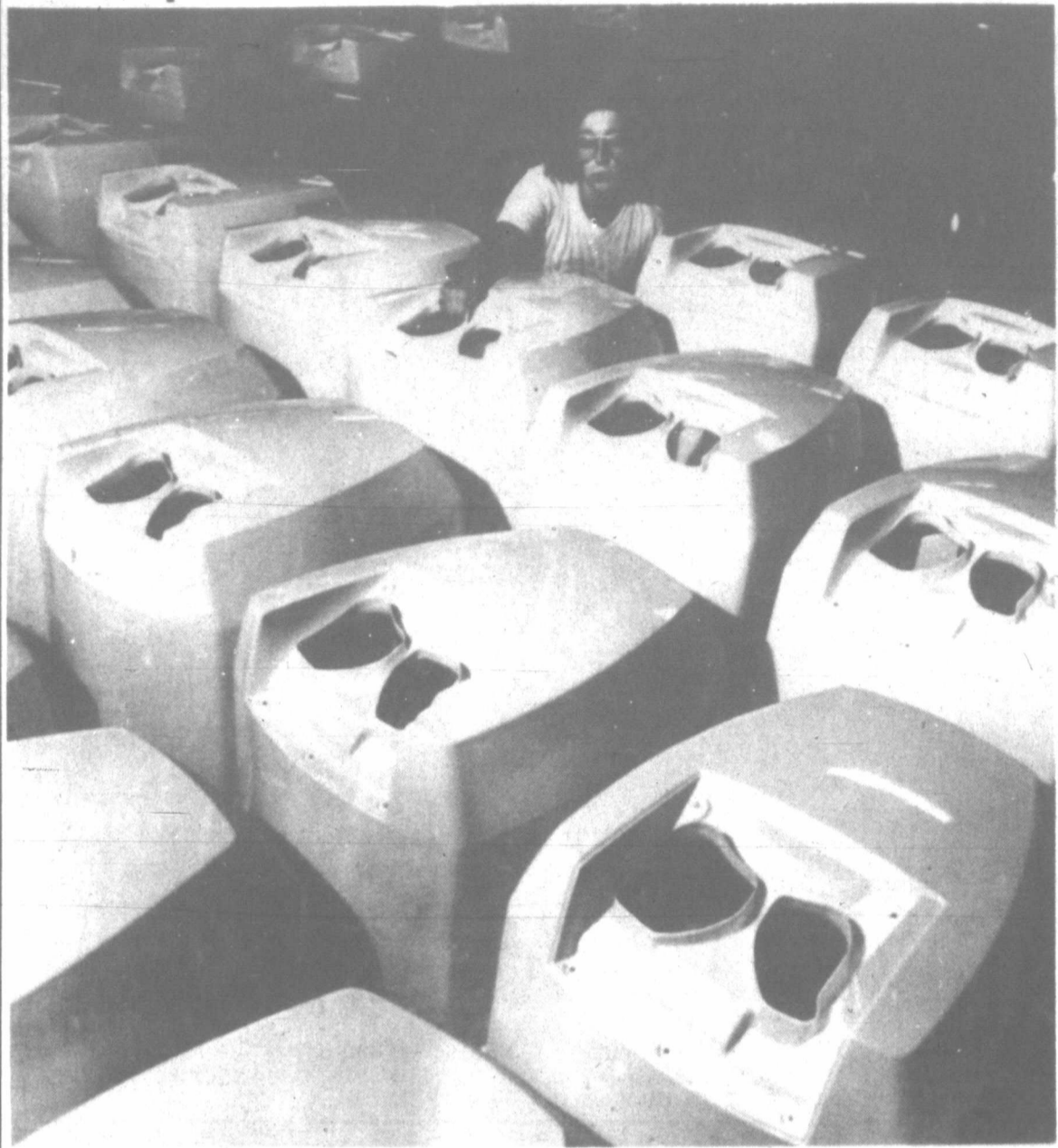
Nancy Hall, decaler at the Outboard Marine Corp. plant in Calhoun, Ga., checks covers on 200-horsepower motors before applying decals. The company says it reached plan-
