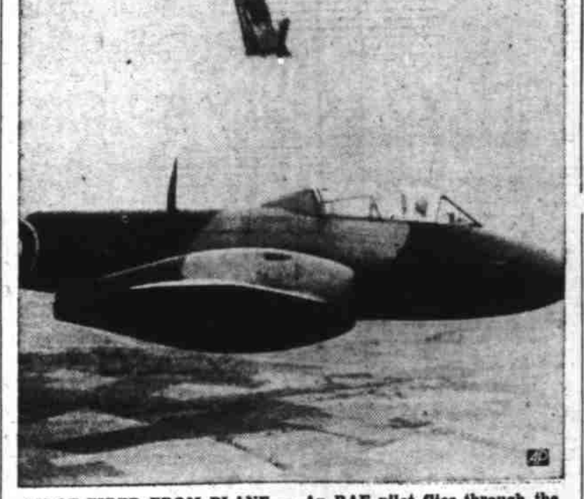
RAF FIRED FROM PLANE — An RAF pilot flies through the air on his pilot-ejection seat at 60 feet a second after being thrown from his jet plane by a cartridge which, when fired, tosses him and his seat from the plane.
