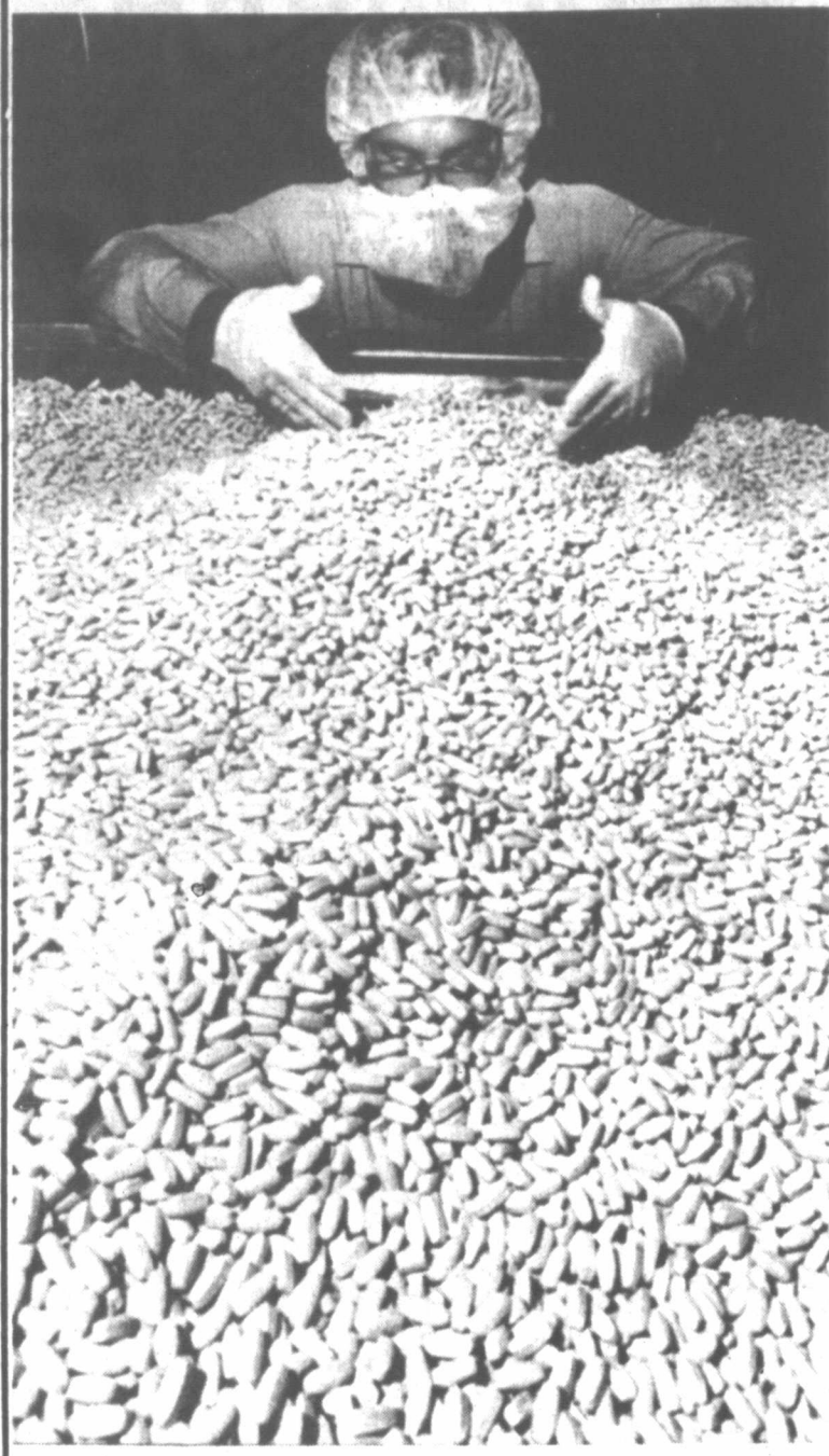
Mitch Russell, operator at Lederle Laboratories' Pearl River, N.Y. plant, examines a pan of vitamins after they've been coated. More than 4.7 million Centrum-brand vitamins are coated every day. Lederle produces more than 1.5 billion Centrum vitamins a year.
