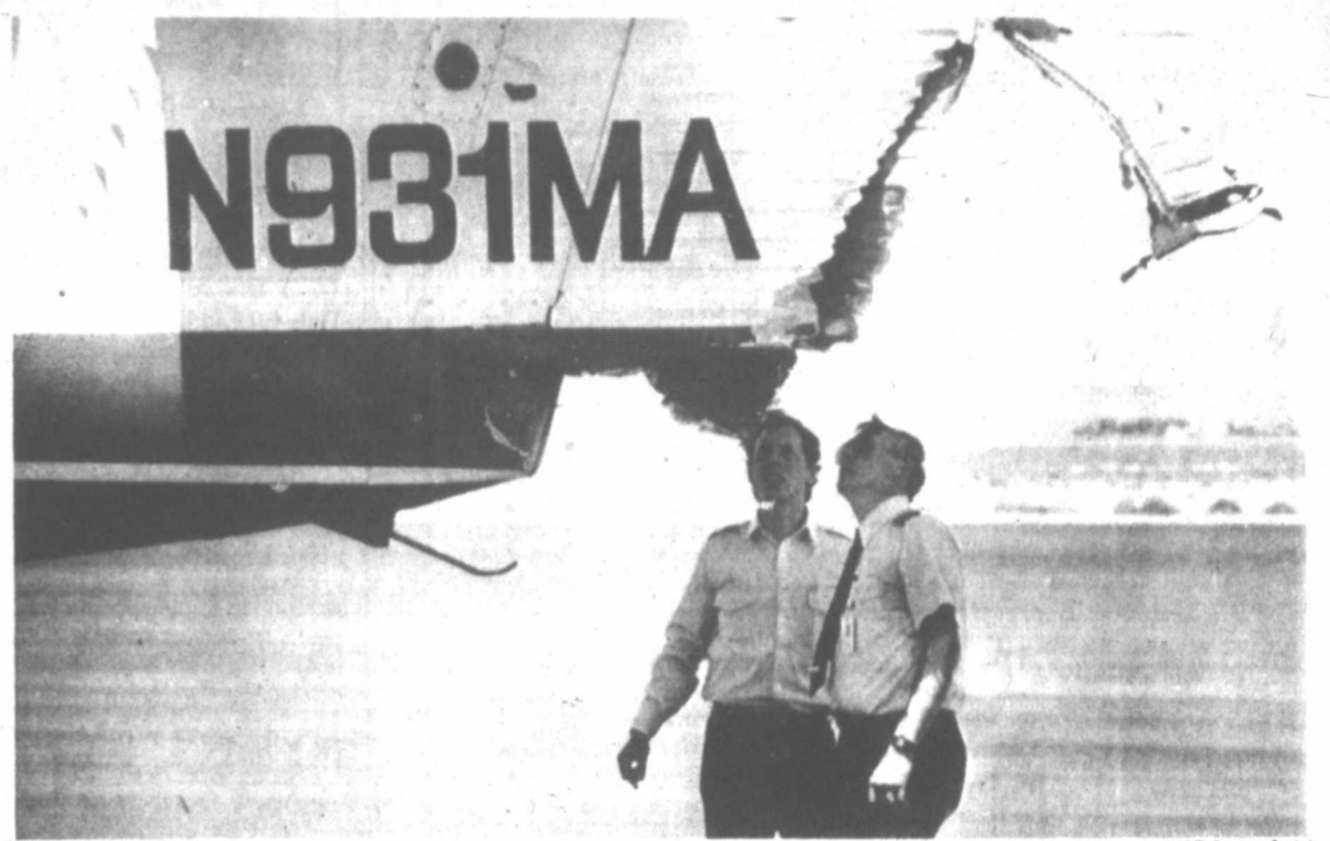
Observers check damaged tail section of DHC-6 aircraft.
