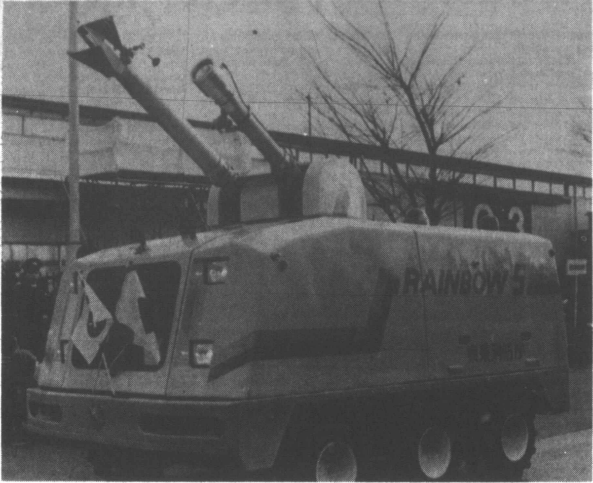
The Rainbow 3, an unmanned firefighting vehicle, makes its debut recently in Tokyo. The computerized wireless-guided vehicle, developed by Tokyo Metropolitan Fire Department, is capable of spraying five tons of water and three tons of fire extinguishing foam per minutes.
