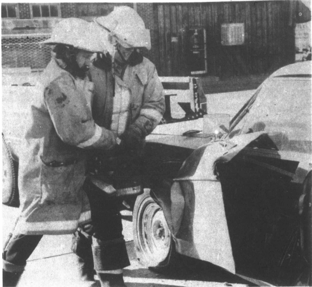
JAWS OF LIFE — Pampa firemen Melvin Irvin and Wayne Smith show how a Jaws of Life hydraulic device can tear open the door of a junked car during an equipment test. The device can apply 5,000 pounds per square inch of pressure on a vehicle and is used to help rescue people pinned in motor vehicle accidents. (Staff Photo by Cathy Spaulding)
