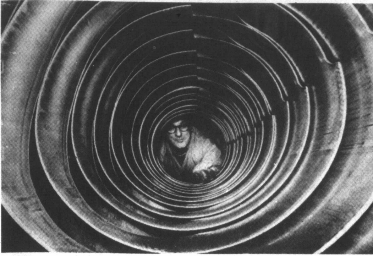
WELDS SNOW SHELLS — Harry Johnz, welder at John Deere in Horicon, Wis., inspects snow blower shells. The shells, used in heavy-duty, two-stage snow blowers, house the augers that pick up the snow before it's blown away by a blower fan. Heavy-duty blowers have 5-10 horsepower engines and clear widths of up to 32 inches. (AP Laserphoto)
