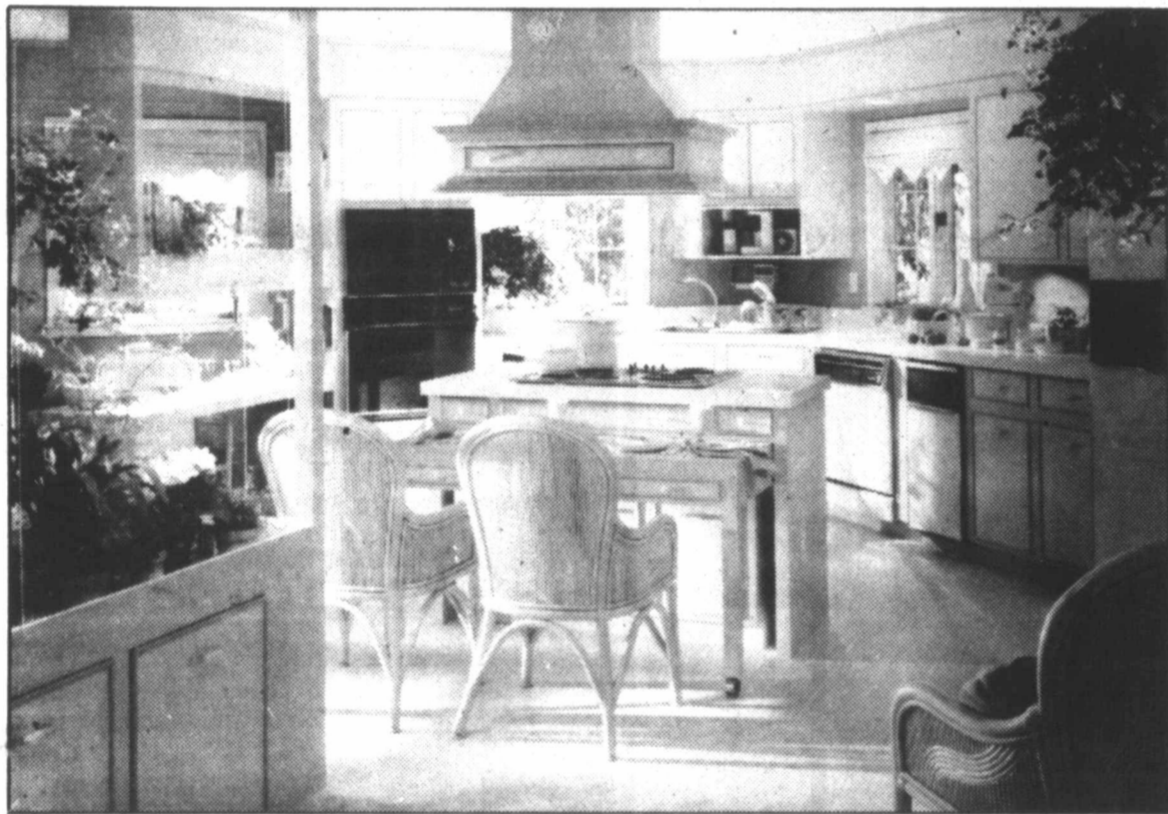
EFFICIENT KITCHEN MODEL —This kitchen is the model of efficiency since the addition of an island unit which is only three or four steps away from the sink and every major appliance. The island has a cook range on top, storage cabinets below and a pull-out table on rollers.
