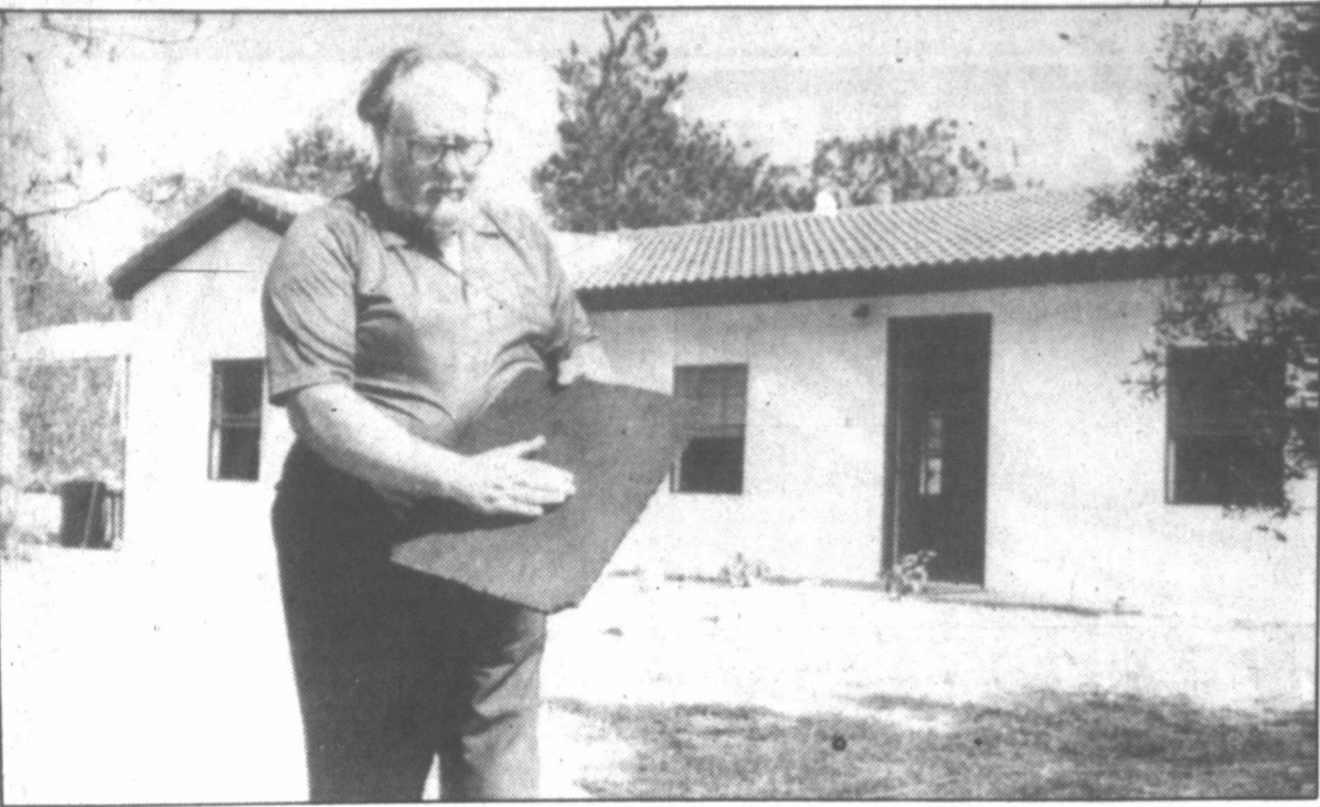
HOUSE OF ASH — Robert Oldham, chairman of King's Bow Inc., shows that a panel made from ashes is cool enough to touch minutes after a blow torch was applied to the other side to demonstrate insulating properties. The material was used to build the prototype house behind Oldham in Navarre, Fla. (AP Laserphoto)
