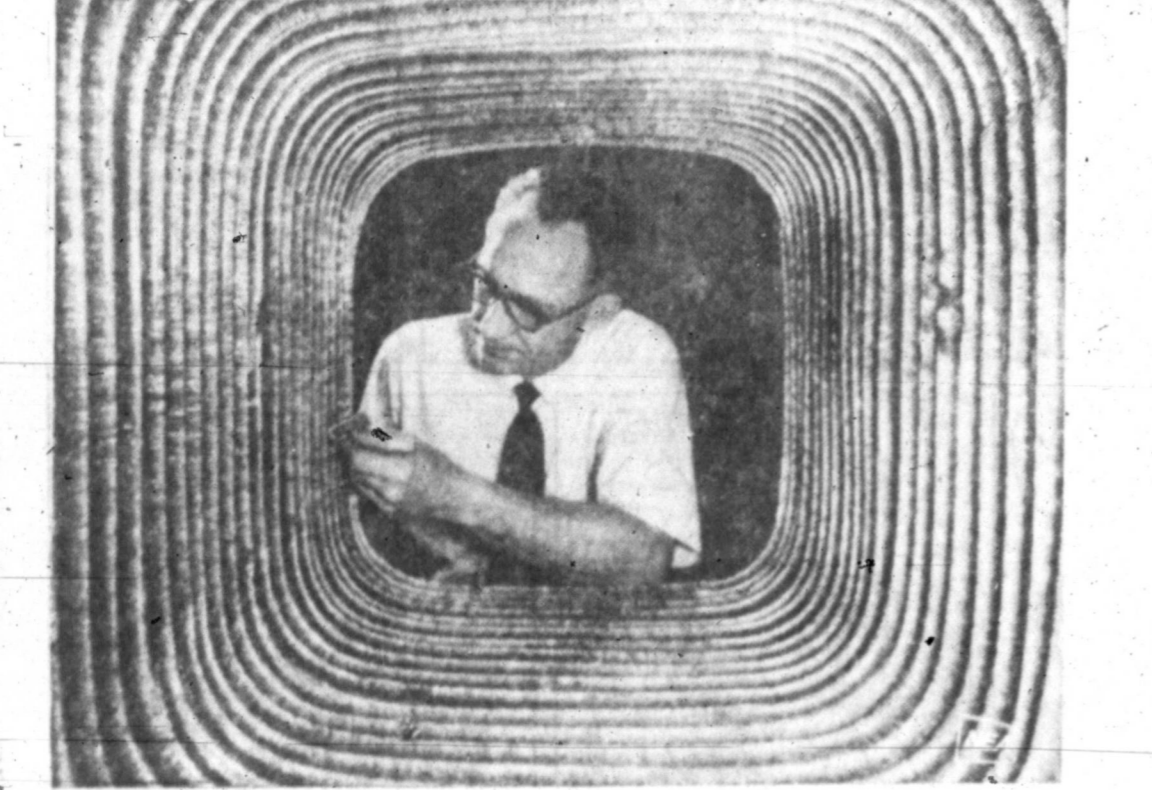
COILED TO STRIKE at heat. Cooling coils of a 10-ton commercial air conditioning system contain more than 1,200 spine fins per inch. Aluminum spine fins wound around refrigerant tubing provide 50 per cent more effective heat dissipation than previously used heat transfer surfaces, according to GE engineers.
