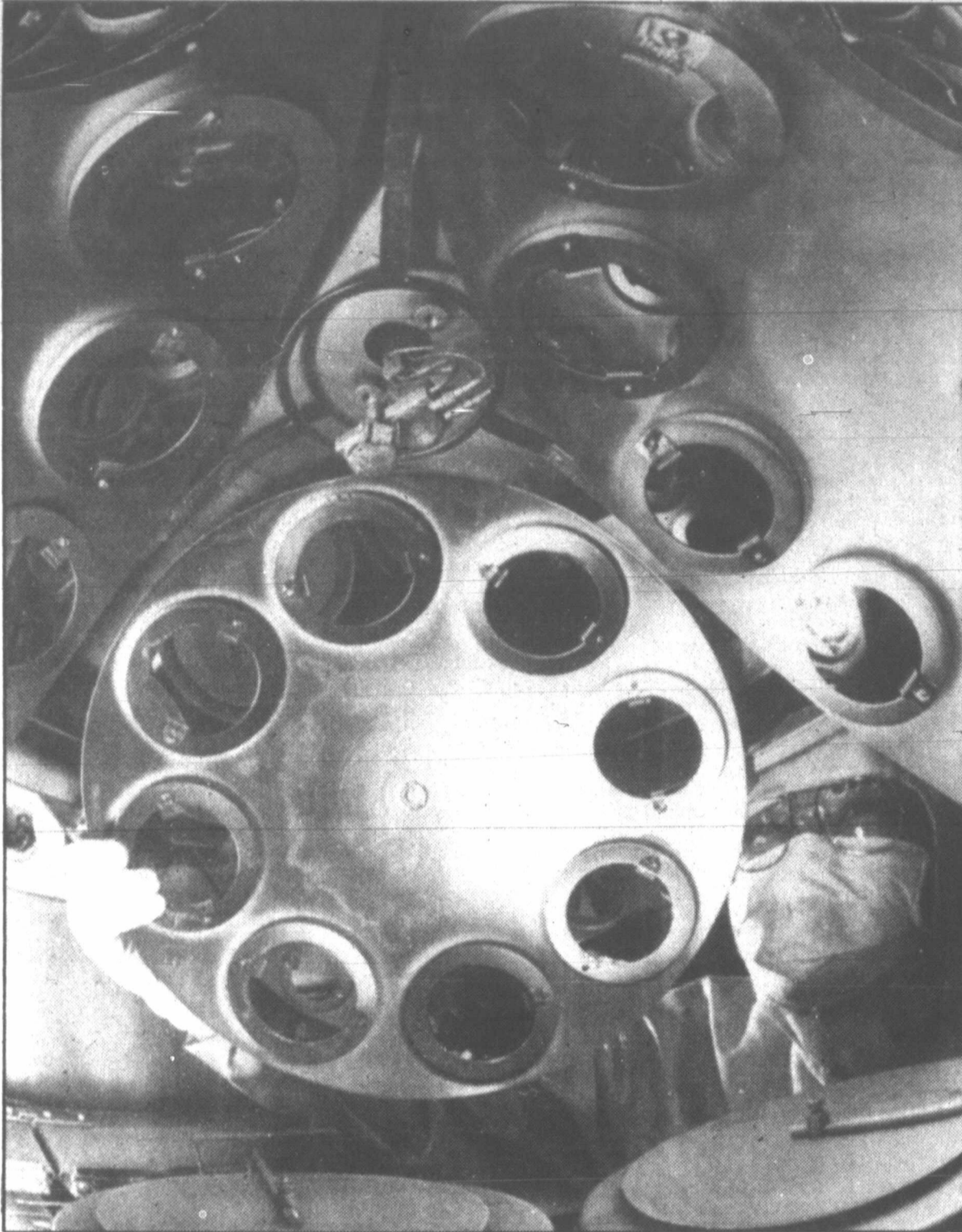
WAFER COATER —A technician loads ceramic wafers into a machine designed to coat each wafer with insulating alumina oxide at Storage Technology Corporation. One wafer produces 380 read-write heads, tiny elements that read and write computer data on a magnetically-coated disk, much like the needle on a record player. Thin film heads make it possible for one StorageTek Disk Drive to store as much information as 40,000 home computers.
