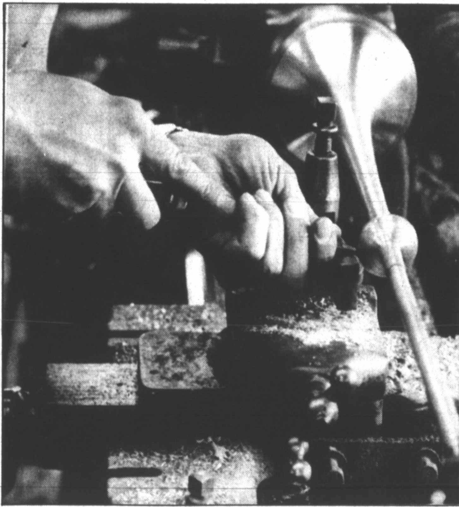
DETAIL WORK —At the lathe, Collier shapes a ferrule on the tube of the baroque trumpet. He first saw one of instruments when he was 14. "I would love to make one of those," he said. The 40-year-old craftsman grew up in Tuscaloosa, Ala., and has been interested in music and metal work since childhood.
