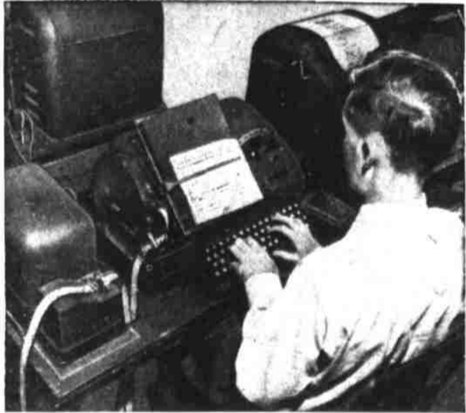
PUNCHER —The operator types copy on this machine. Note the device to the left of his left hand which punches holes in the tape and the machine on the far left which produces the wire signals by which the hole-pattern can be duplicated in another tape at a distant point. Just above the operator's head, the copy is being reproduced on a typewriter in the short lines which will make even lines of type when the tape is fed into a line caster. The device beside the copy above the operator's right hand measures the space each letter will take.
