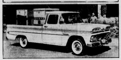
A revolutionary new suspension system gives wast improvement in ride, durability, and control to 1960 Chevrolet trucks. Front wheels are independently sprung on frictionless torsion rods. Rear suspensions are new, with coil springs on light-duty models and stronger, softer riding
