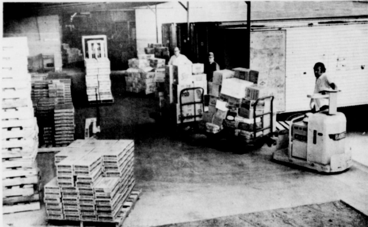
CUTTING OUT THE MIDDLE MAN is made possible in the new JRB Distribution Center by the use of these mechanical tuggers and numerous carts plus the use of pallets and fork lifts. In this manner, merchandise is moved quickly and economically to JRB Stores and to the customer.
