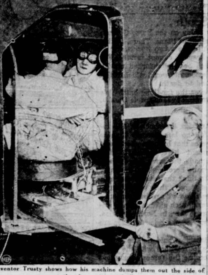
Inventor Trusty shows how his machine dumps them out the side of the plane, seats and all.
