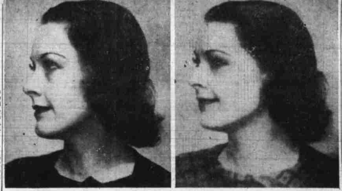
STILL-CAMERA PHOTO TELEVISED IMAGE These unretouched photographs show the detail held in television by the new 441-line transmitter.
