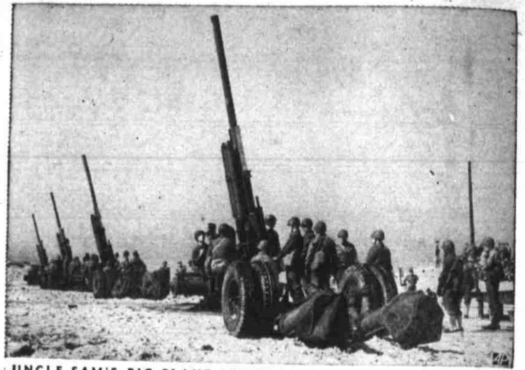
UNCLE SAM'S BIG PLANE BUSTERS —A battery of 90-mm. anti-aircraft guns, heaviest used by the U. S. Coast Artillery for defense against planes, gets a workout in the field. These guns can be get up ready to shoot in 13 minutes, are manned by a crew of 15 and fire 18 rounds per minute. They are now in use in North Africa, the Solomons and on other United Nations fronts.
