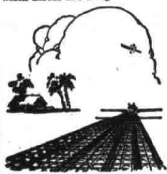
It consists of steel linked plates perforated for traction. Each strip is ten feet long and 15 inches wide and is linked together to form a runway 150 feet wide by 3,000 feet long.
