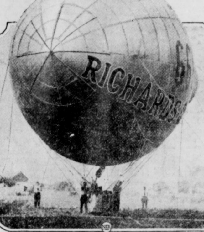
The smallest dirigible ever built, less than 40 feet long, recently made a second trial flight at Wright Field, Dayton, O., and was proclaimed a success by army and civilian engineers. A four-cylinder motorcycle engine propels the craft, which weighs 700 pounds and carries a load of the same weight.
