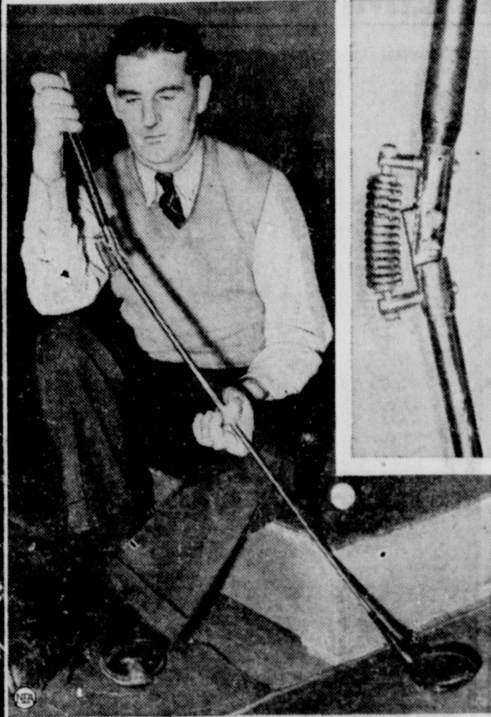
John Homans, professional of the Riverside Golf Club of Weston, Mass., exhibits his new swing corrector club, bent as the result of an improper swing. Inset is the spring just below the grip which is opened by a false move.
