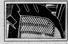
This heavy, broad, traction and non-skid tread is held to the cord body of the tire with Two Extra Layers of Gum-Dipped Cords, a patented construction, making the cord body and tread an inseparable unit.
