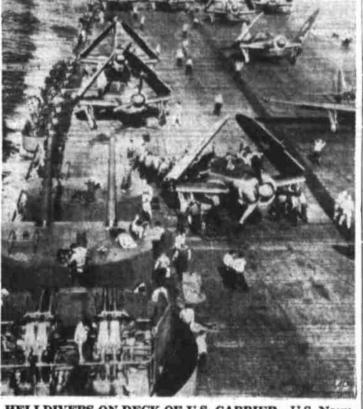
HELLDIVERS ON DECK OF U.S. CARRIER-U.S. Navy Curtiss Helldivers are spotted on the deck of this U.S. carrier. In foreground, left, is a 40mm. battery and immediately beyond are two 5-inch gun turrets. In the gallery at side are Marines and their 20mm weapons.
