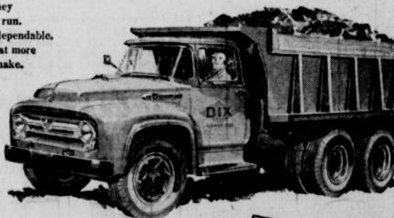
Ford's rugged T-800 is a real money-maker! Choose from two heavy-duty V-8's, developing 200 and 212 horsepower. Both are equipped with sodium-cooled exhaust valves that last as much as five times longer! Power steering and tachous eter standard at no extra cost.
