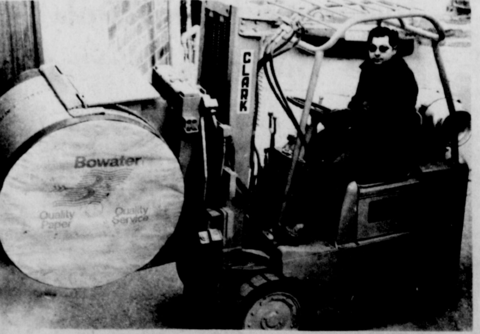
Eastland Telegram employee Kenneth Rawson demonstrates one of the newest pieces of equipment at the Telegram. The fork lift is used to unload and store rolls of paper which arrive by truck for use in printing the papers. Each roll weighs an average of 1000 lbs. (Photo by Steve Haines)
