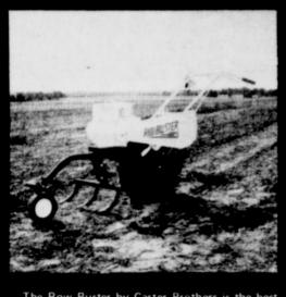
The Row Buster by Carter Brothers is the best designed garden plow on the market today. It is well built and rugged to give dependable service for many years. Standard features include a tractor grip tire that can be filled with water for better traction; belt and chain drive; both horizontal and vertical adjustments of the front wheel and a powerful engine with reduction gear. The adjustable plow footing fits all standard garden plow kit attachments and allows for plowing depth
