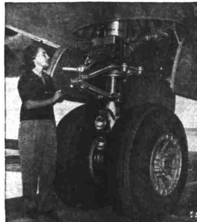
AIR ENGINEER — Miss Jane Little inspects the forward landing gear assembly she designed on the Globemaster C-124 transport at Douglas Aircraft plant, Long Beach, Cal.
