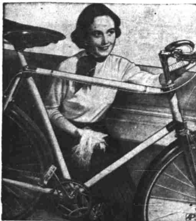
GLASS BICYCLE — Anne Giles holds a Bicycle Show exhibit in London and a piece of glass fibre from which frame is built. Makers claim it's stronger than steel and much lighter.
