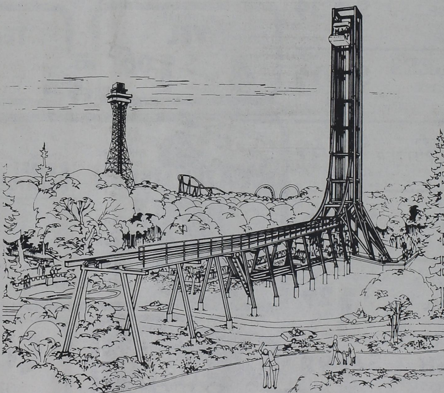
TEXAS CLIFFHANGER--The world's first total freefall ride, the Texas Cliffhanger, will open in late April at Six Flags Over Texas. Riders will be dropped at freefall speed from the top of the 128-foot-tall tower. Passengers will end up riding flat on their backs as the ride's computer-controlled brakes bring the gondolas to a stop.
