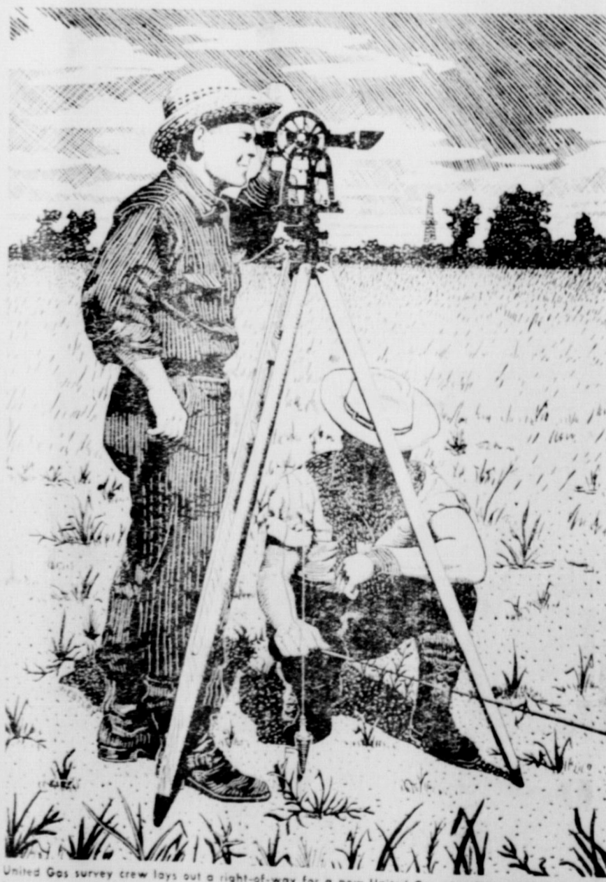
United Gas survey crew lays out a right-of-way for a new United Gas pipe line
