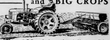
• Full germination, good stands, big crops-all depend on accurate seeding. Case Seedmeter drills measure out seed in a steady flow, uniform in all furrows, at all rates of seeding. Plain and fertilizer types, many sizes. Can be had with grass seeder attachment. All Case drills can be hydraulically controlled.
