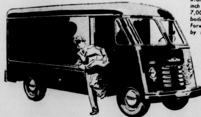
LIGHT-DUTY DE LUXE PANEL* Model 3105—116-inch wheelbase, Maximum G.V.W. 4,600 lb. Also available in Medium-Duty model 3805—137-inch wheelbase, Maximum G.V.W. 6,700 lb.
